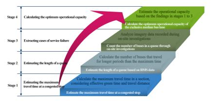
[Figure 42] Four Stages of Calculating Optimum Operational Capacity
