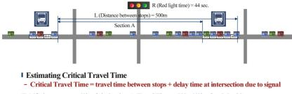
Ex) If a bus moves at 60km/h in Section A, Travel Time = 500m/60km/h x 3.6 = 30 sec. If the expected value is assumed half the red time, 22 sec., the critical travel time is estimated at approximately 52 sec.
